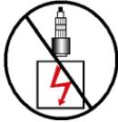
Do not attach sensors to any object with a high potential voltage i.e. a voltage that exceeds 50 V DC or 32 V AC or the 'safety extra low voltage' (SELV) defined by your local power authority.
