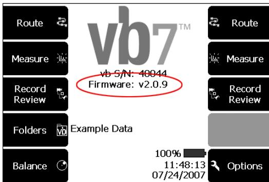
In order to Proflash a vbX series instrument such as the vb7 vibration analyzer, you must first add the instrument to the Ascent software. If you have not done so already, follow the **Add vbX Instrument to Ascent** procedure below. If your instrument has been added
